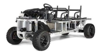
To prevent rust and ensure long life, look for vehicles built on rustproof, corrosion-resistant aluminum frames (shown above).
